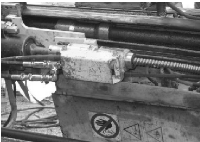
Fig. 2 Drilling and grouting adapter on drilling feed unit
